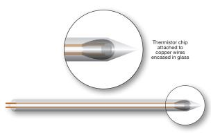
CDN's ProAccurate® Quick-Read® pocket thermometers use thermistor sensors with new and innovative technology. The sensor is located in the tip. When inserted only one half of an inch, it will provide an unusually accurate and stable response in 6 seconds or less.
